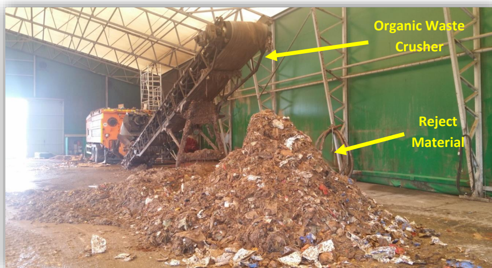
Figure 1: Organic waste crusher and reject material at the Organic Site
